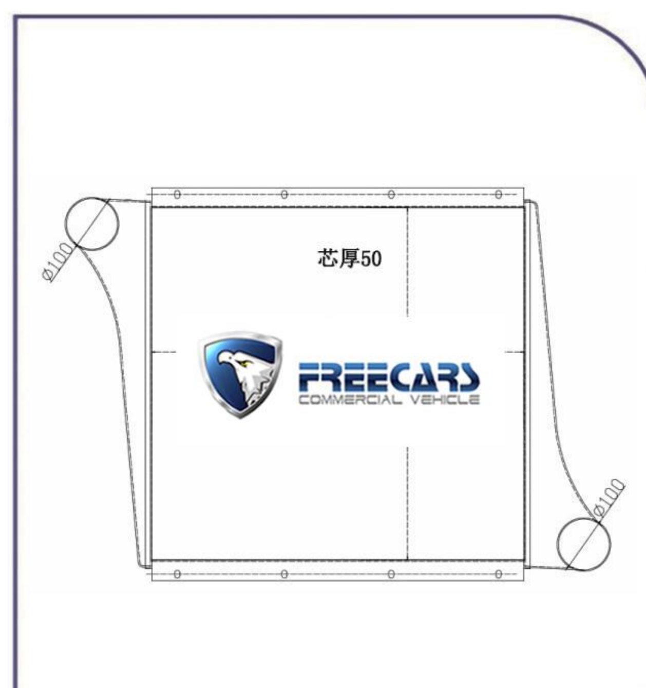
SACT-09 CORE SIZE:730*692*50 APP: SINOTRUK OEM:WG9725530020
